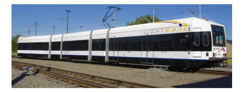
In 1999, Kinkisharyo began delivering 73 of North America's first 70% low-floor LRVs to New Jersey Transit, spurring the redevelopment of an urban area where now ridership demands are greatly increasing. By adding two additional sections to the existing 3 Section LRVs, the new 5 Section LRV increases rider capacity by 50%. Kinkisharyo was awarded the 5 Section contract in 2014. **Formation:** 8 - Axle Articulating
