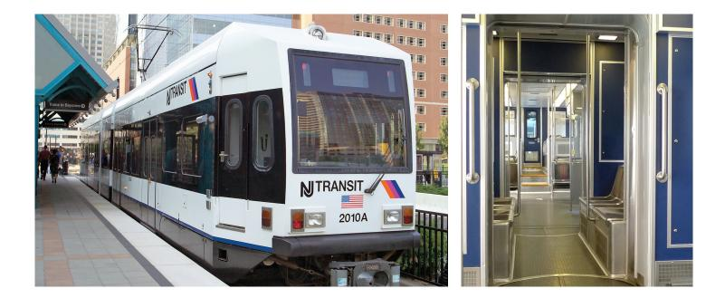
KINKISHARYO's 1st 70% low-floor LRV with a crash energy management carbody and a streetcar clearance envelope. With performance rivaling rapid transit and reliability exceeding the industry standard, the Hudson-Bergen Low-Floor LRV set a new standard for LRVs in North America. **Formation:** 6 - Axle Articulating
